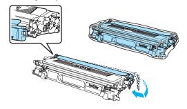
8 Hold the green parts of the belt unit with both hands and lift the belt unit up, then pull it out.
